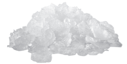
WET GRANULAR ICE 25% RESIDUAL WATER CONTENT
